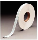
for sterilisation facilities to ensure that products have been exposed to the sterilisation process. Labels turn from blue to pink after exposure to 121°C for 3-10 mins, or 134°C for 0.5—2 mins. **Catalogue No. AC986**
